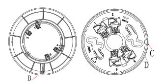
The sounder base does not require cabling. It will share the termination of the detector.
