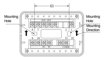
IN+, IN-: Input cable from previous device, IN+ is positive, and IN- is negative.
