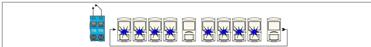
Self-tests every 7 h. Self-test and remote self-test failure: 4 blue flashes
