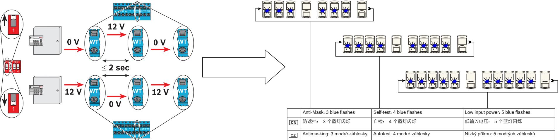
Trouble Memory: Pulse WT input to recall last trouble condition from memory. Pulse WT input again to clear memory. When memory is recalled, it automatically clears after 12 h.
