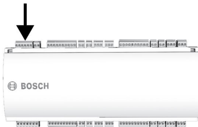
Figure 4.7: Interface for internal power supply
