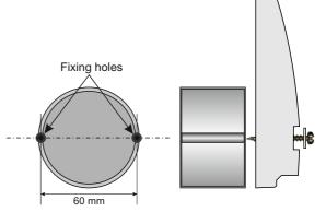
To **lock the housing** press in one of the enclosed seals at the bottom. The housing cannot be opened without destroying the seal.
