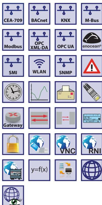
The LGATE-902 Gateway is a powerful gateway that can host user specific graphical pages. The gateways provide connectivity functions to concurrently integrate CEA-709 (LonMark Systems), BACnet, KNX, Modbus, and M-Bus. Local operation and override is provided by the built-in jog dial and the backlit display (128x64 pixels). Device and data point information is provided by the web interface and shown on the display via symbols and in text format.
