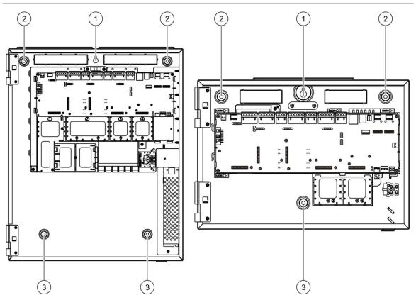
Figure 7: Mounting hole locations
