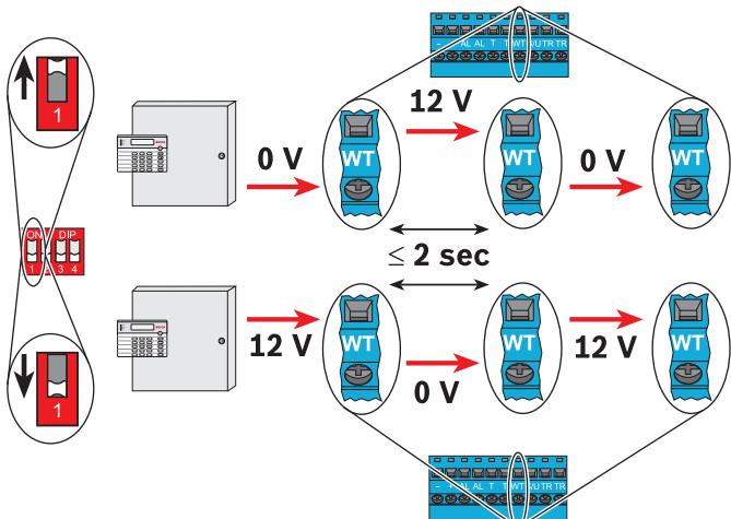
Trouble Memory: Pulse WT input to recall last trouble condition from memory. Pulse WT input again to clear memory. When memory is recalled, it automatically clears after 12 h.
