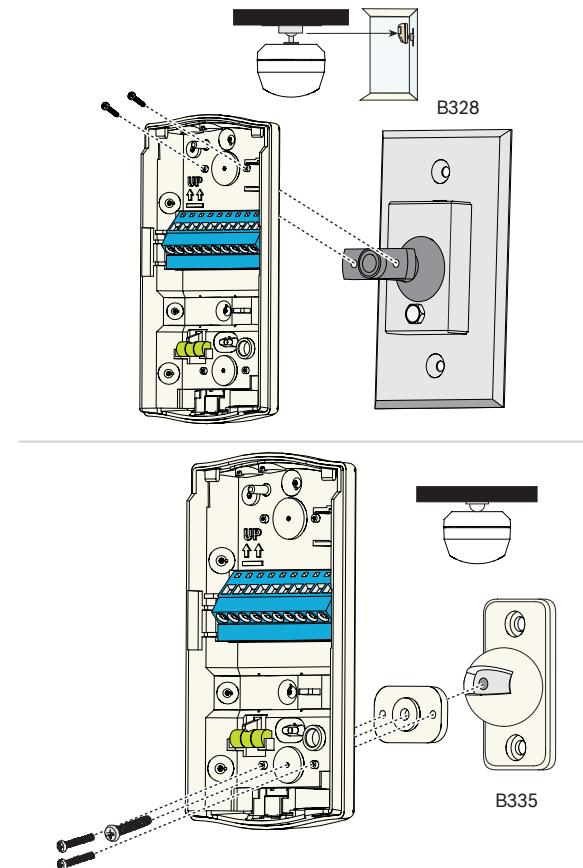
**US** A mounting bracket can reduce the detector's range and create dead zones.
