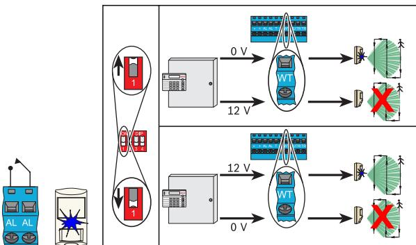
**Remote Self-Test:** Remote Self-test automatically occurs when walk test changes from disabled to enabled (change in terminal voltage).
