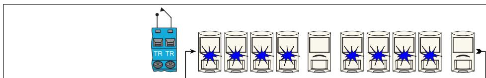
Self-tests every 7 h. Self-test and remote self-test failure: 4 blue flashes
