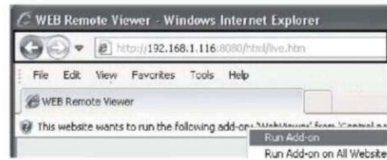
1. Open the browser and enter the IP address of DVR, or enter the URL address in the address bar.
