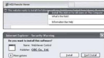
3. Click the upper warning bar to install the ActiveX before enabling the add-in function.
