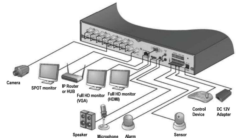
! Since the cable quality may affect directly to the video quality depending on the distance between the camera and DVR, it is recommended to consult an authorized installer when installing the DVR.
