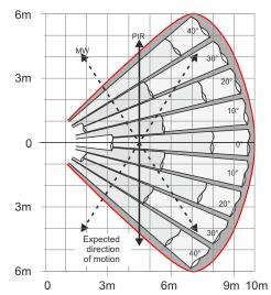
Vertical detection coverage, vertical inclination 7° downward
