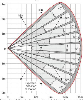
Due to the additional microwave, the dual detector has a very high detection capacity even with diagonal movement.
