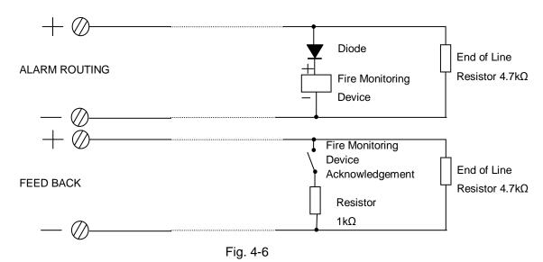
A  $4.7k\Omega$  resistor is connected at terminal ALARM ROUTING and FEED BACK as factory default. Please remove it and keep it well before connection. Connect the loop in correct polarity and add the resistor to the end of the line.
