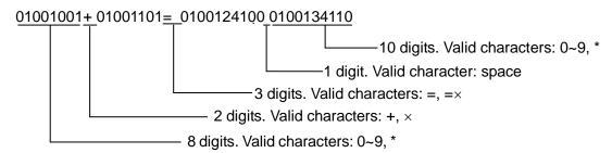
The meaning of the above equation: If point smoke detector No. 010 in Zone 010 or point smoke detector No. 011 in Zone 010 alarms, sounder strobe No. 012 in Zone 010 will start immediately, and sounder strobe No. 013 in Zone 010 will start after 10x10 seconds delay.
