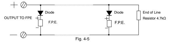
A  $4.7k\Omega$  resistor is connected to the terminal OUTPUT TO FPE as factory default. Please remove it and keep it well before connection. Connect the loop in correct polarity and add the resistor to the end of the line.
