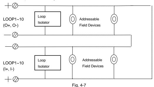
Note: If more than 32 devices are connected to the loop, loop isolators shall be used and each loop isolator shall not cover more than 32 detectors.
