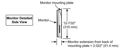
Figure 11: Rack mount hardware reference with 18.5" monitor
