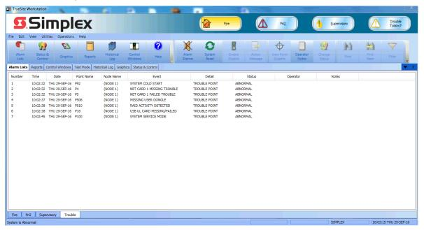
Figure 8: TrueSite Workstation sample alarm lists screen
