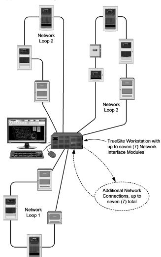
Figure 6: Typical Interface of Multiple Network Loops Using a TrueSite Workstation Server
