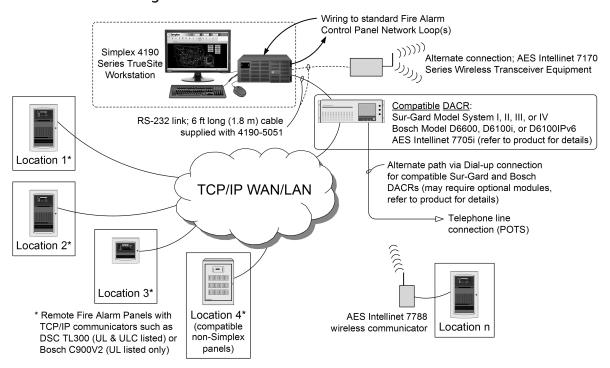
Figure 7: DACR interface reference diagram
