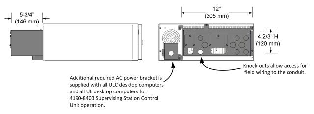
Figure 12: Rear mounted mechanical protection - conduit entry bracket enclosure reference (required for ULC listing)
