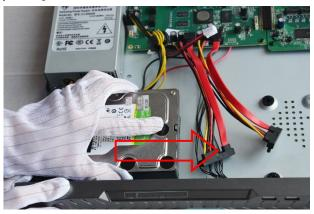
Step 6 Turn the device over, and fasten the rest two hard disk fixing screws, as shown in Fixing the hard disk.
