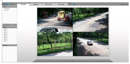
The main screen provides the functions of live video viewing, video playback, alarm search, quick setup, camera configuration, and NVR configuration. For details, see the *Network Video Recorder (NVR) User Guide*.
