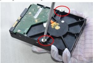
Step 5 Route the hard disk fixing screws through the holes on the base, push the hard disk to the appropriate position according to the direction of the arrow, as shown in Inserting the hard disk.
